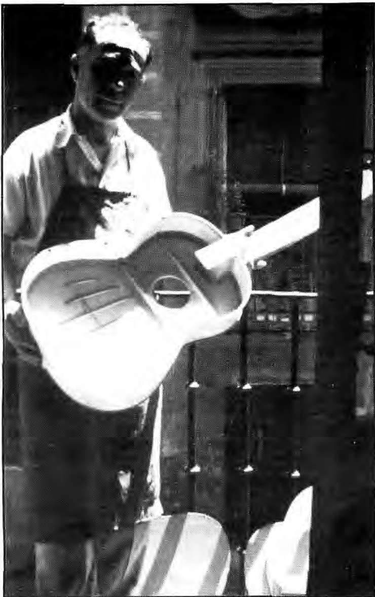
MARCELO HOLDING A GUITAR WHICH IS READY FOR THE BACK TO BE GLUED IN PLACE.
